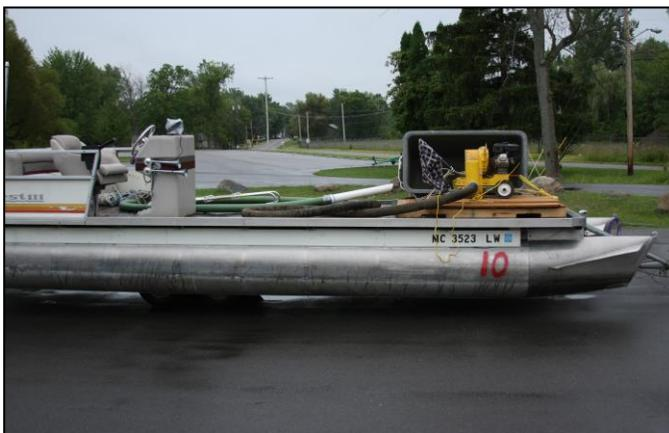
Figure 42. A DASH boat for hand-removal of milfoil or other nuisance vegetation. ©Restorative Lake Sciences, LLC
